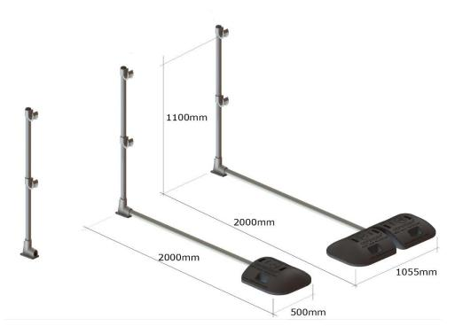
Lay out the equipment in approximately the positions shown below. Always ensure that you and the equipment are at a safe distance from the roof edge. It is recommended that this distance is no less than 2m.
