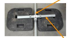
As with the single counterweight insert the locking collar into the first hole. The solid bar then passes through the locking collars until it is visible in the second hole. The short tee is positioned on the solid bar between the 2 counterweights. The setscrew on the locking collars is then tightened and the setscrew on the short tee is tightened. The 1575mm tube is then placed into the short tee and the other end into the base of the post and the setscrews tightened.
